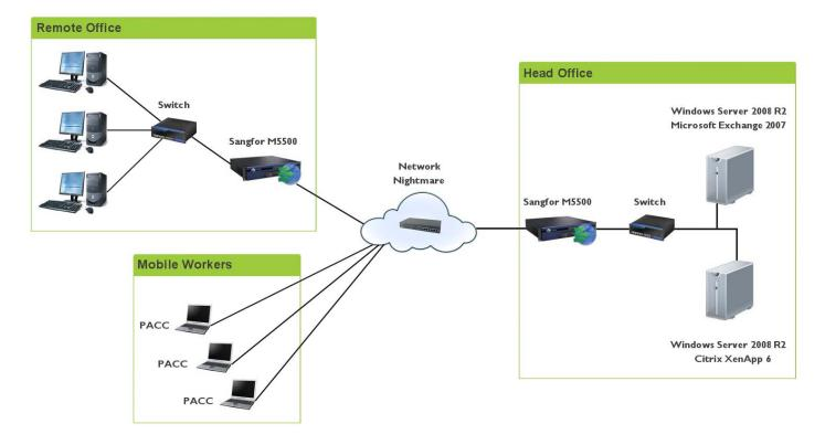
For performance testing we created a network in the lab to simulate an environment comprising a head office and remote site. Two WANACC M5500 appliances were used with one placed in front of the head office network and the other at the remote site.
