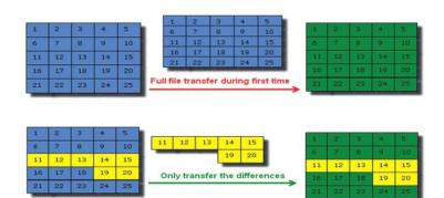
WAN optimisation appliances are designed to accelerate these applications using a wide variety of technologies. At its foundation, the technology removes the need to transfer redundant data over WAN links. Appliances are placed on each side of the WAN connection where they examine the data being passed over the link and cache it in local stores.
