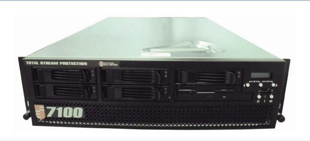
Physically, the TSP 7100 delivers an impressive hardware specification as it has a Newisys 4300-E enterprise class server as its foundation. The 3U chassis is very well built and designed and delivers the full range of fault tolerant features we would expect to see at this level of the security appliance market. A quartet of 2.2GHz AMD Opteron 848 processors are in the driving seat and these are partnered by a total of 4GB of DDR400 ECC SDRAM memory split equally between all four processors.
