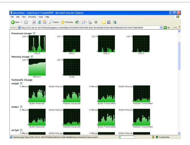
The TSP 7100 real-time monitor display, showing the system under test. The processors are easily handling the traffic load, and in spite of high memory utilisation the system has still not needed to use the swap file.
