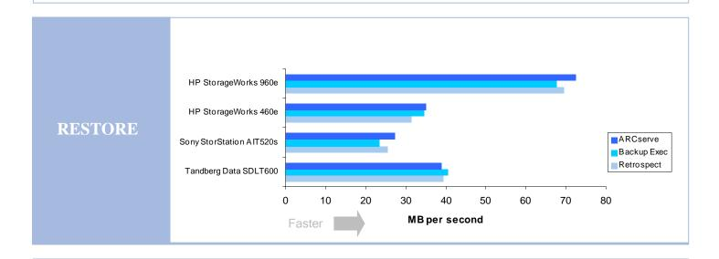
In general, all three products returned similar results for the data restoration tests although ARCserve, once, again proved to be marginally faster that the rest. With the HP StorageWorks Ultrium 960, ARCserve returned 72.4MB/sec which was 4 per cent faster than Retrospect and 7 per cent faster than Backup Exec. The smallest margins came with the Tandberg Data SDLT600 with all three products returning restoration speeds of between 39MB/sec and 40.5MB/sec.
